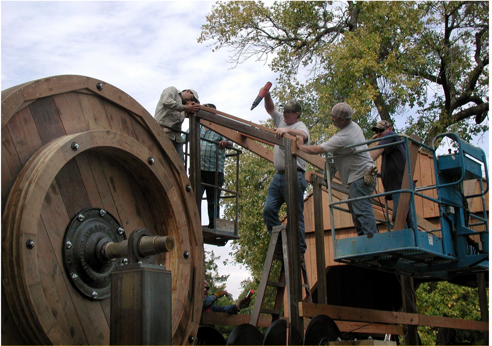
The huge wooden band wheel was built from scratch using original iron fittings.
