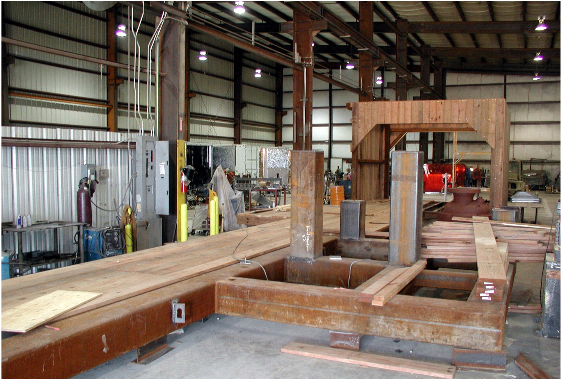
The derrick deck and engine house are constructed with steel frames at the indoor shop of SMC, a Bartlesville firm that built the derrick.
